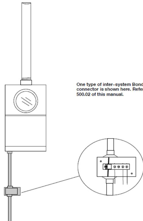
One type of inter-system Bonding connector is shown here. Refer to Section 500.02 of this manual.
