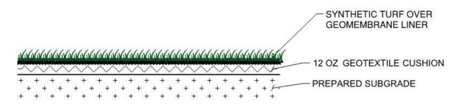
Ameren Missouri is considering using an engineered synthetic turf system at Labadie CCR unit closures, depending upon the ease of constructability and design performance experienced at LEC.
