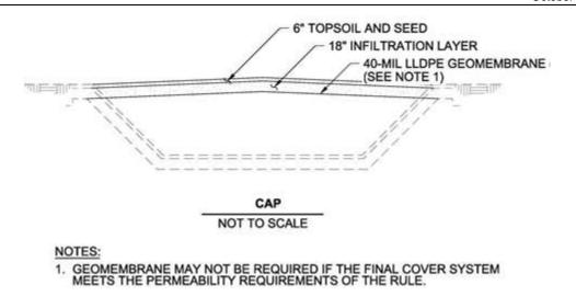
Figure 1: Typical CCR Unit Cap
