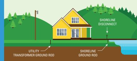
In order for your docks electrical system to function in a safe manner, the grounding system must be connected all the way back to the utility transformer. This is accomplished by testing the grounding system between the dock and the house panel box, not to the ground rod or shoreline disconnect near the seawall. This test should show that there is less than 1 ohms resistance on the grounding system.
