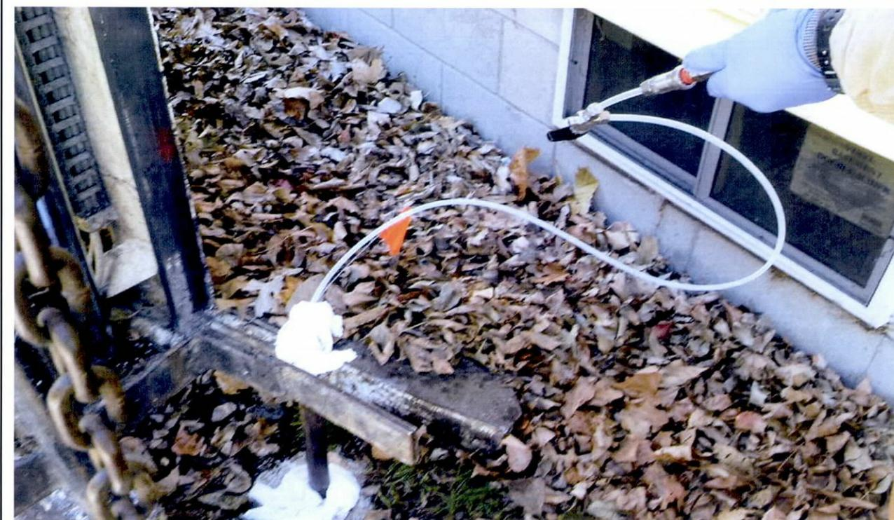
Photo 16: 506-E-7-Soil Vapor Purging
