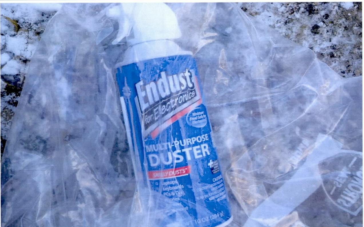
Photo 22: Leak Detection Compound (Duster Spray containing 1,1-Difluoroethane)
