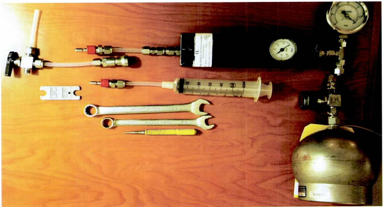
Photo 26: Soil Vapor Purging and Sampling Assembly with Summa Can
