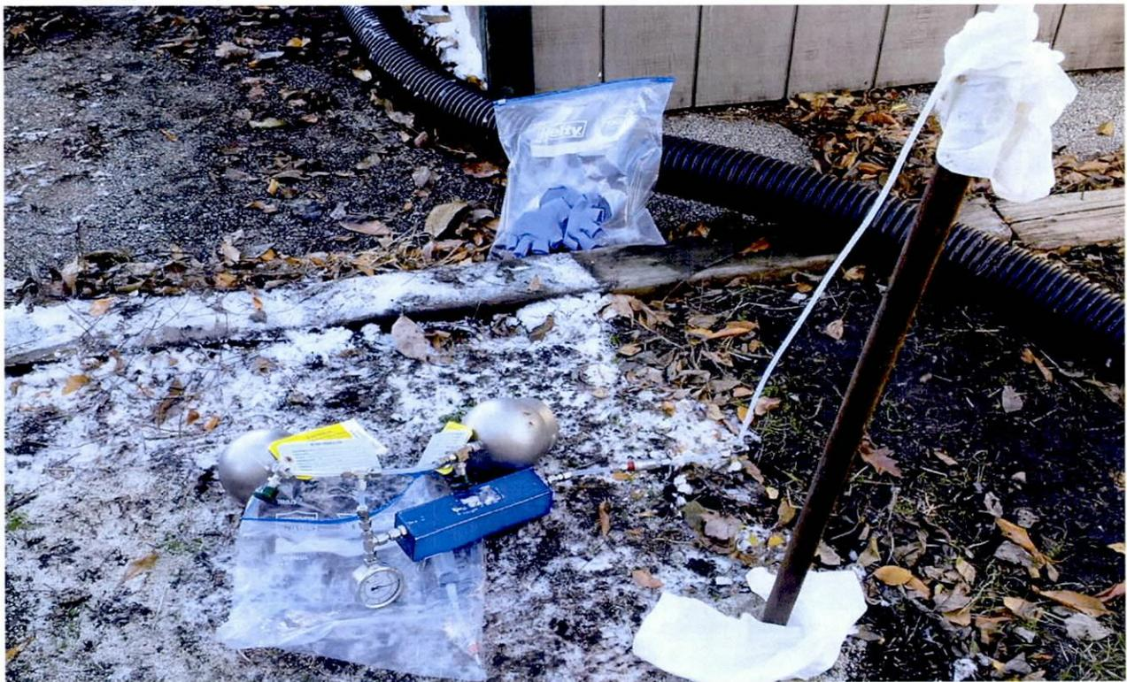
Photo 21: 508-N-9-Soil Vapor Sampling with Duplicate
