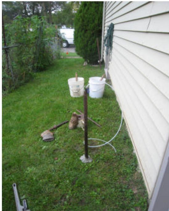
**PHOTO 2: View to North along west side of 505 E. Washington at location of VP505EWASH-2. Probe in ground, tubing inside probe.**
