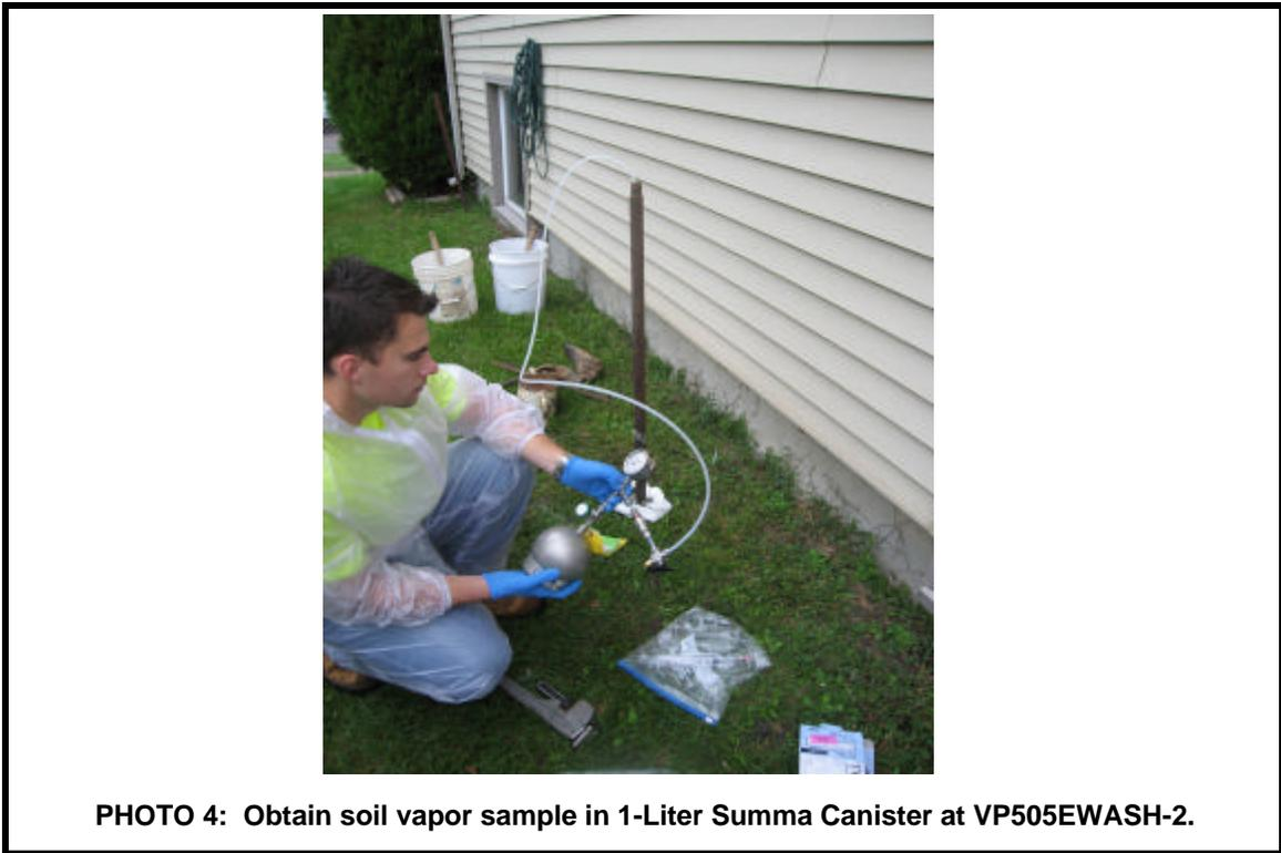
**PHOTO 4: Obtain soil vapor sample in 1-Liter Summa Canister at VP505EWASH-2.**
