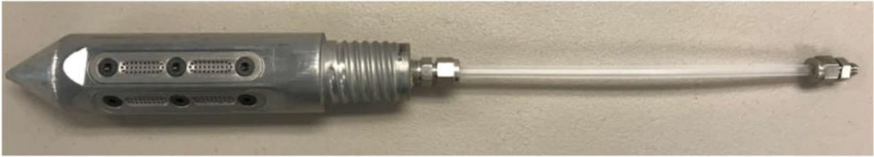
6. Gently pull on the reducer after the fittings have been attached to make sure that it is attached properly. If the fittings are over tight then the FEP can snap; if they are too loose than the FEP can pull out of the fitting.
