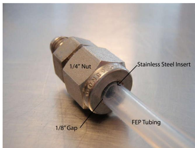
5. For the other end of the FEP, slide on another 1/4” SwageLok® nut and 1/4” nylon ferrule. Insert the end of the FEP into a 1/4 “to 1/8” SwageLok®
