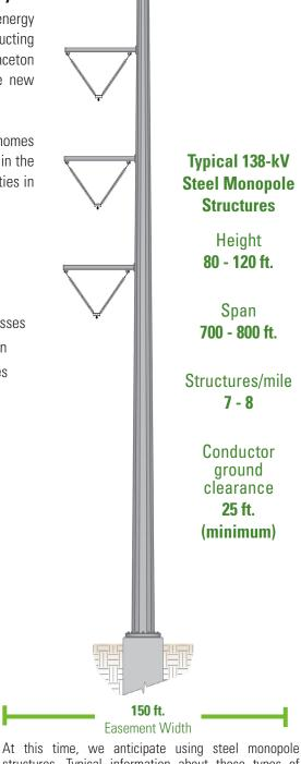
structures. Typical information about these types of structures is provided above. Note: This graphic is not to scale, and the number of arms on a typical structure may vary depending on the final route.
