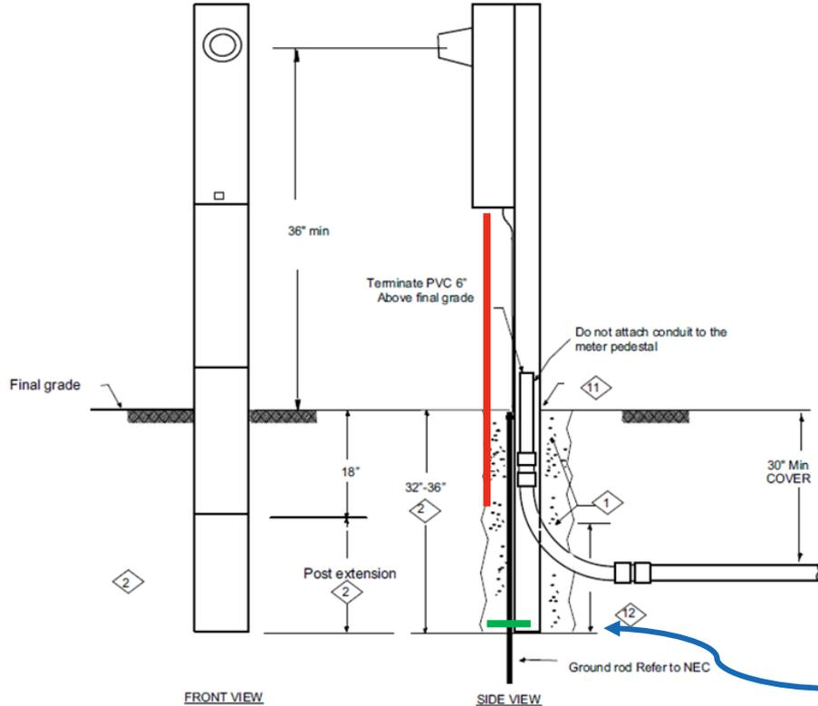
Backfill with tamped, crushed rock including entire conduit elbow
