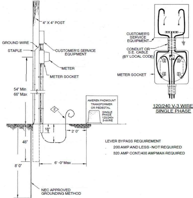
This figure showing mounting of equipment represents both individual components and that of a meter / main combo unit approved for temp. service.
