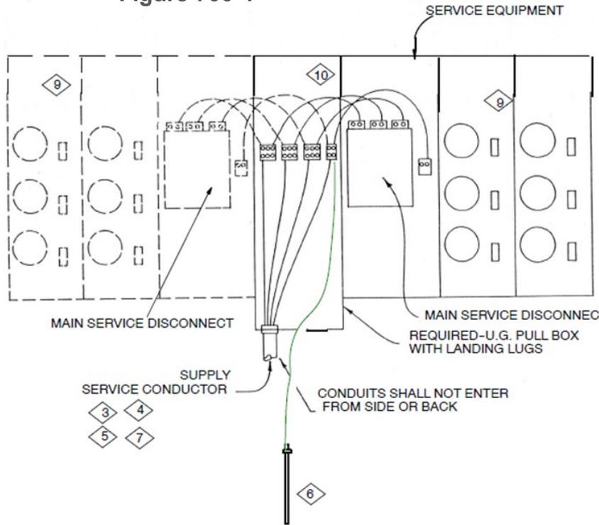
Route supply side conductors so they have some slack to compensate for freeze / thaw movement
