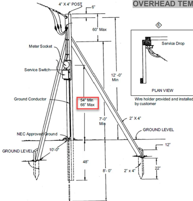
1. Install the temporary connection in a manner suitable for transfer to the permanent location.
