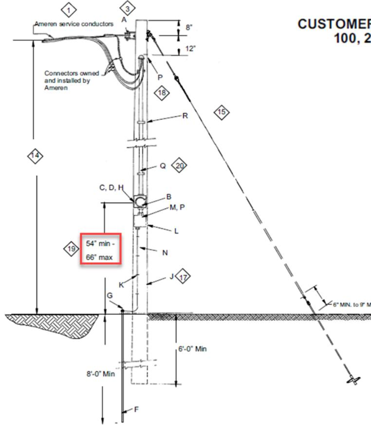
**CUSTOMER OWNED PERMANENT OH METER POLE INSTALLATION**
