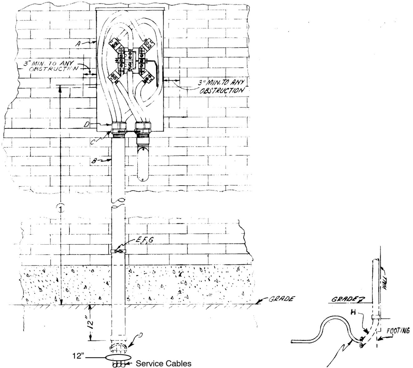
NOTE: Loop indicate slack in the cables, allowing for settlement.
