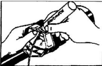
12. Lubricate the filling tube on the bladder section.
