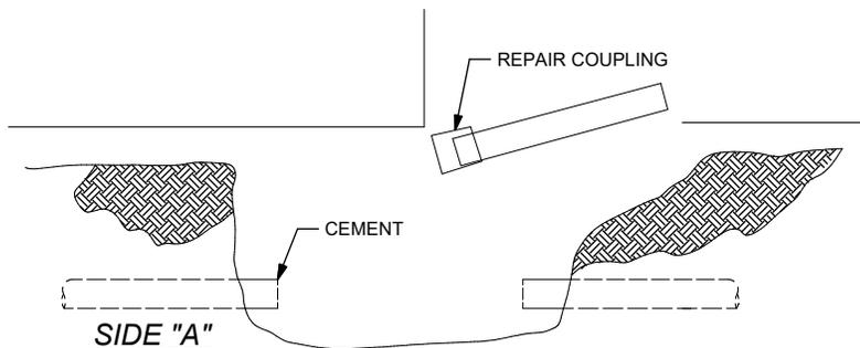
4. Apply a liberal amount of cement, coating the entire length of the socket, and install coupling on repair length and apply cement to side "A". Slip the conduit into the socket with a firm twist until bottom is felt, holding the joint motionless for 15 seconds longer when the weather is very cold. Do not drive or twist a complete joint. Full curing takes one hour.
