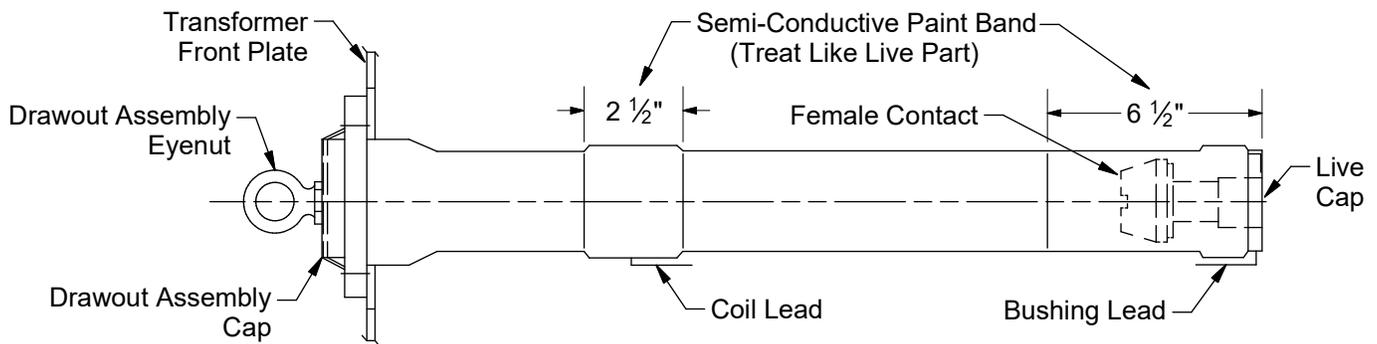
**Figure 1 - Loadbreak Dry Well Fuseholder Housing**
