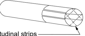
3. Apply circumferential wraps of plastic tape over the longitudinally applied tape.
