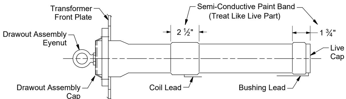
**Figure 2 - Non-Loadbreak Dry Well Fuseholder Housing**
