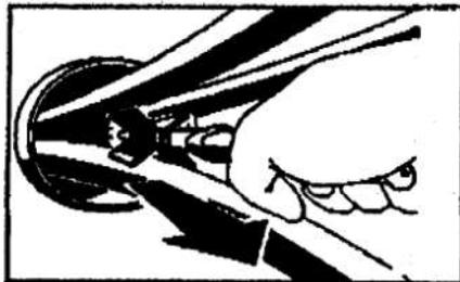
5. If applicable: Remove tie wraps from the cable bundle. Spread cables. Remove clip core and sealant as much as possible with a pair of pliers
