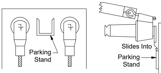
3. Attach the feed-thru bushing eye and crossbar firmly to shotgun tool. Slide the feed-thru bushing onto parking stand. Tighten down eye by rotating shotgun tool clockwise until snug. **DO NOT OVERTIGHTEN.** See Figure 3. **NOTE: #14 ground wire not shown.**
