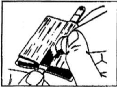
4. Remove one protection paper and lubricate abundantly the larger surface of the clip wing.
