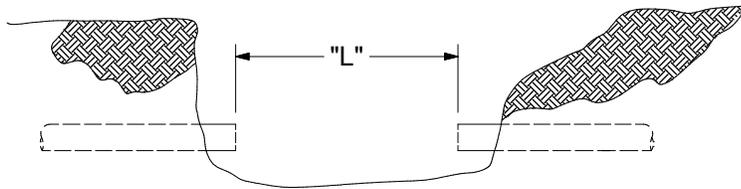
3. Measure and cut repair piece  $\frac{1}{2}$ " shorter than "L" (see table). Clean all edges to be fitted
