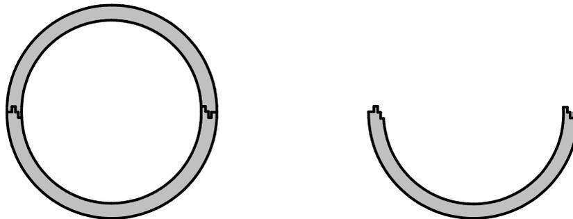
End View of Split Conduit Interlocking Design
