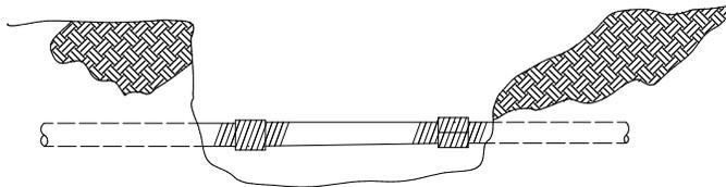
8. Completely seal repair sleeve or coupling with 1-1/2" wide plastic tape.
