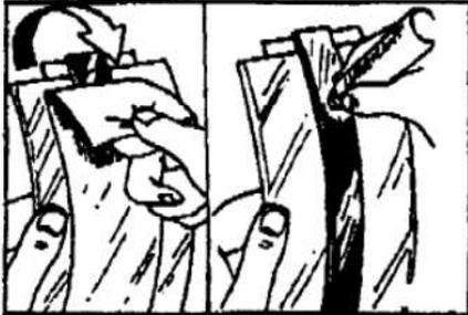
10. Remove the protective paper from the outside of the sealing strip and lubricate abundantly.
