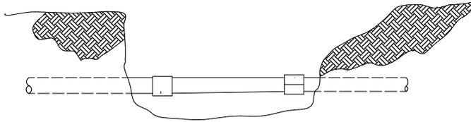
7. Apply cement to joint and slide repair sleeve OR both halves of split repair coupling over joint.
