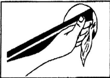
1. It is recommended to wet clean the duct and cable Sheath. Remove as much dirt, crust, mud, etc. as possible. **For ducts with 3 or more cables, continue with step 2. For 0, 1, or 2 cables skip to step 9.**
