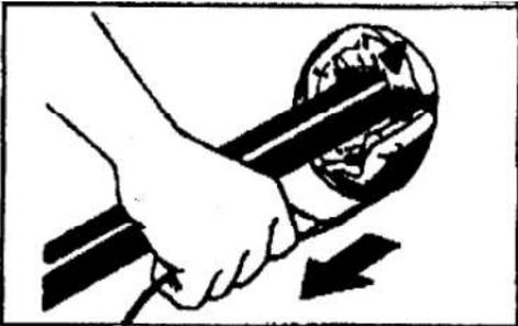
17. BEFORE removing the installation tool connection from the filling tube, pull out of the filling tube in one gentle move in the direction of the cable installation to complete.
