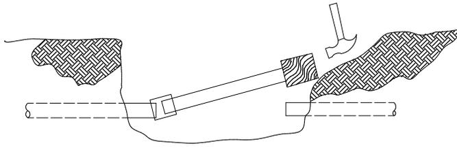
5. Use hammer block to drive repair piece into place.
