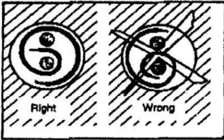
14. In case of two cables, wrap bladder around the cables as shown starting with the largest cable.
