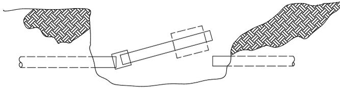
6. Slide repair sleeve on conduit past joint.
