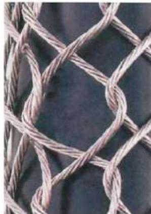
3. At the very end of the mesh grip, twist the lacing ends tightly together. Wrap the ends tightly around the tail of the grip once or twice. Excess lace can be cut off.
