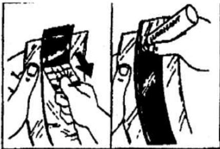
11. Continue with lubrication of the inside of the sealing strip.
