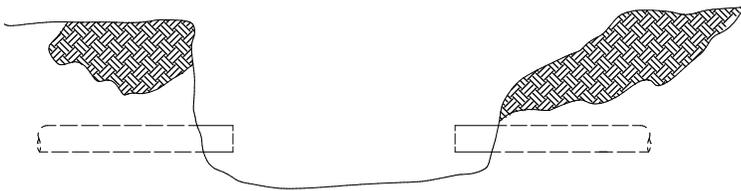
2. Square cut edges, making sure that male ends have an inside beveled edge.
