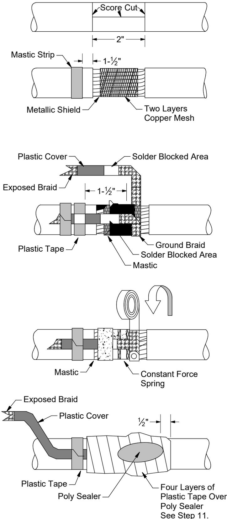
1. Score jacket carefully as shown. Do not cut through concentrics, which are #18 AWG wires. Remove the jacket by prying and lifting along score. Cut.
