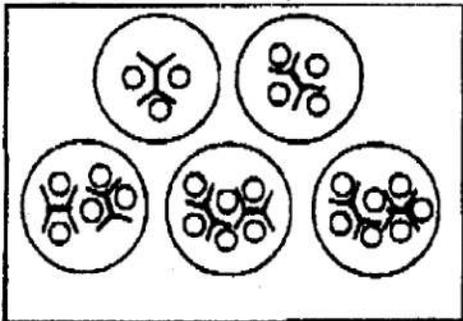
2. Examples for different multiple cable configuration. One RDSS-Clip can seal up to four cables. If more cables are to be sealed, use one extra clip per three additional cables.
