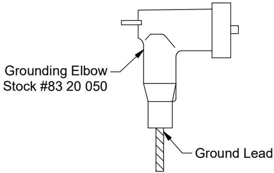
1. Connect lead on Grounding Elbow to Ground. **IMPORTANT: DO NOT INSERT GROUNDING ELBOW INTO FEED-THRU BUSHING UNTIL CIRCUIT HAS BEEN TESTED "DEAD".** Grounding elbow shown in Figure 1.
