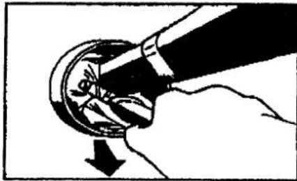
4. Pull the bladder out of the duct with a pair of pliers.
