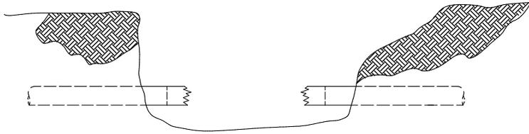
1. Expose conduit and clear debris, cleaning surfaces to be joined and eliminating cracked or defective parts of conduit.
