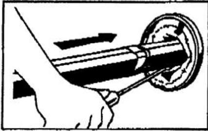
2. Release bladder from the cable or cable bundle.
