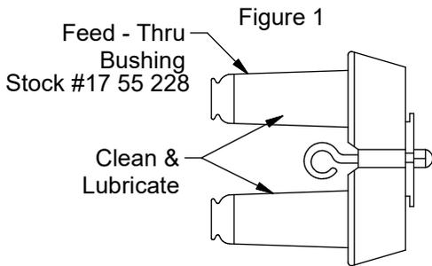
2. Remove protective covers from the feed-thru bushing. Clean and lubricate the surfaces of the feed-thru bushing with silicone grease. **ALWAYS REPLACE PROTECTIVE COVERS WHEN THE FEED-THRU BUSHING IS NOT IN USE.** Connect one #14 ground wire to grounding point of feed-thru bushing. Connect the other end of the wire to ground, leaving enough slack to operate with a shotgun tool. Feed-thru bushing shown in Figure 2.
