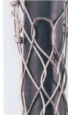
2. Don't pull lacing too tight. Leave a space between adjoining loops approximately equal to the width of one diamond of the mesh grip.
